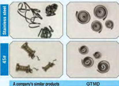
Under the same working conditions, our company's GTMD series grooving inserts have better chip breaking performance, which can reduce the downtime for chip removal.
