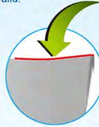
Smooth connection of insert nose and cutting edge makes rake face smoother.
