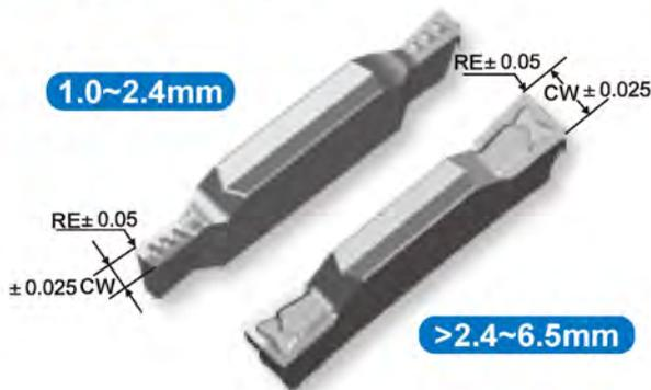
The width of the Little Squirrel series precise grooving inserts can be anything between 1.0mm to 6.5mm, which means products with any edge width or nose radius can be provided according to customers' requirements. The inserts are mainly used for precise grooving, such as sealing slot and locating slot, etc.
