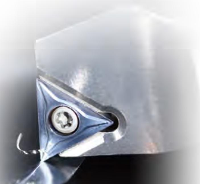
**Corresponding tool holders of insert VC   (Damping tool holder) S-type clamping**
